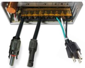
AC Plug Connect to AC wall socket or generator
