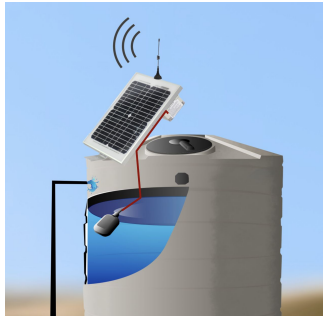
Transmitter at Tank End
